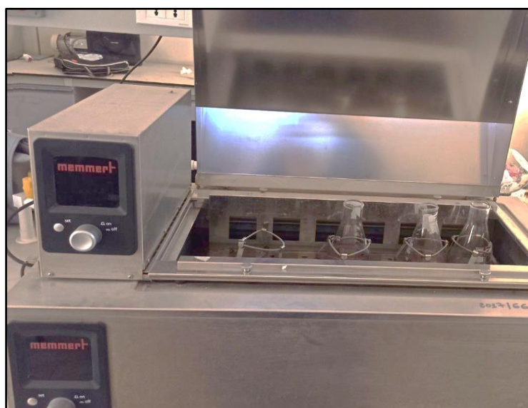
Figure III.12. Image of rotary shaker used for dye adsorption experiments
