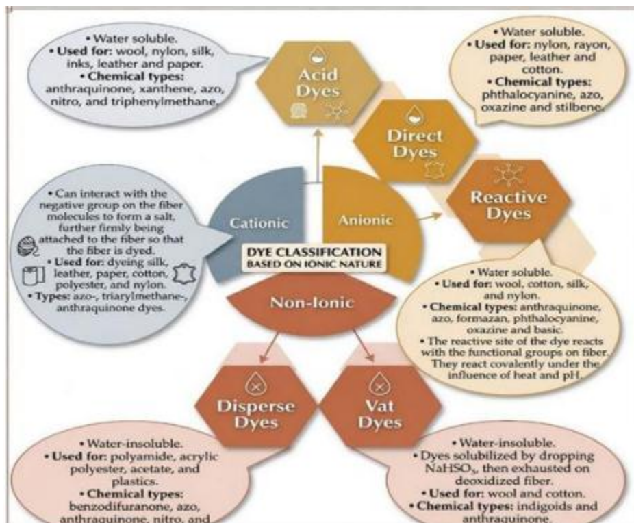
Figure II.2. Classifying dyes according to their ionic structure [24].
