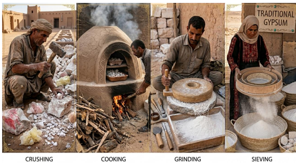
Figure II.7. Stages of preparing gypsum powder using the traditional method [55] .
