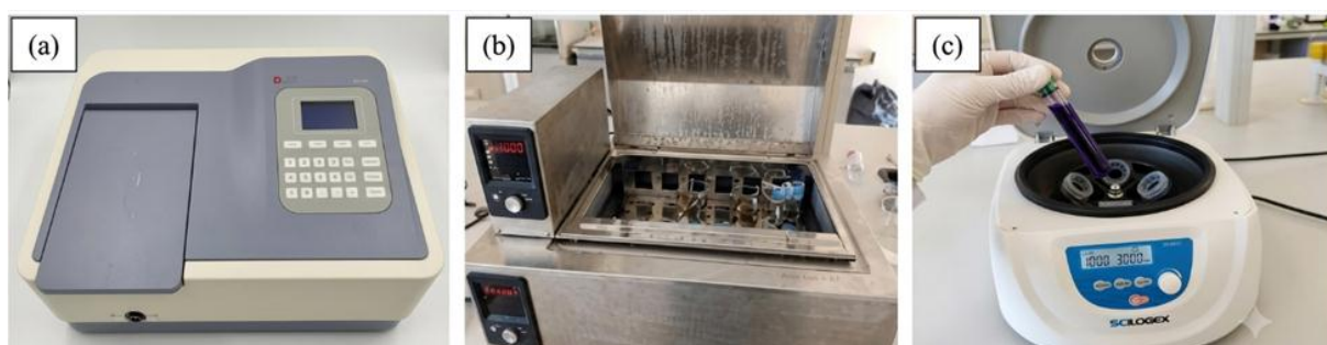
Figure III.12. Photographs of the equipment used for dye adsorption experiments: (a) UV-Visible (UV-Vis) spectrophotometer, (b) shaking water bath, and (c) centrifuge.
