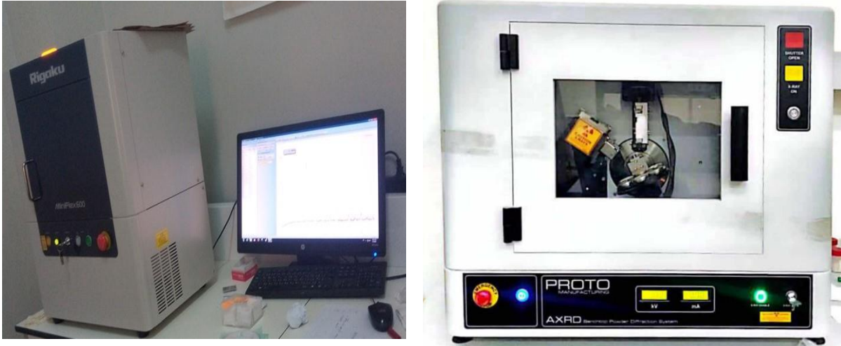
Figure II.3: (a) Diffractometer type (Rigaku-MiniFlex600).
