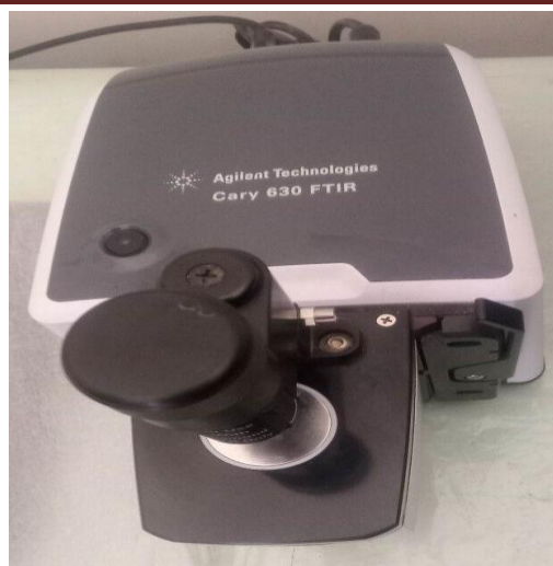
Figure II.8: Fourier Transform Infrared Spectrophotometer apparatus type of Cary 630 FTIR
