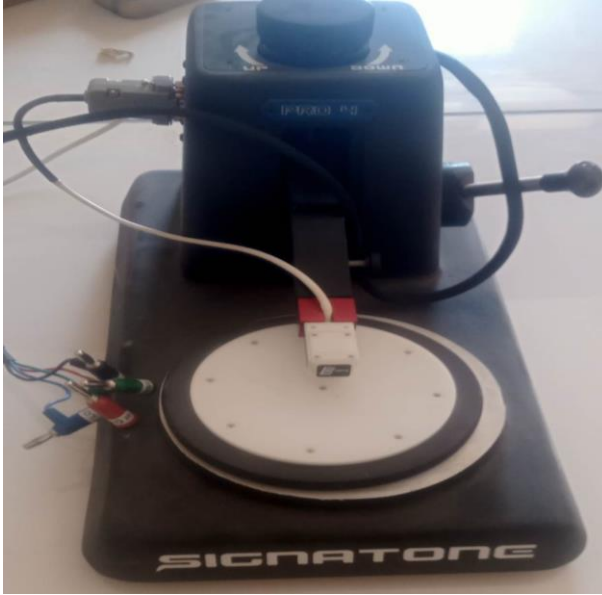
Figure II.15: Four-point device type of Signatone PRO4 Figure II.16: Schematic diagram of a four-point device
