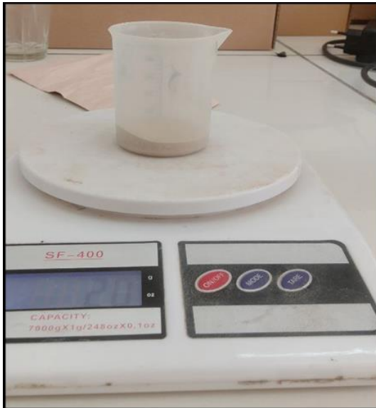
Figure 10: The sample weight 20g of soil (ouada R , Bey A.2024)
