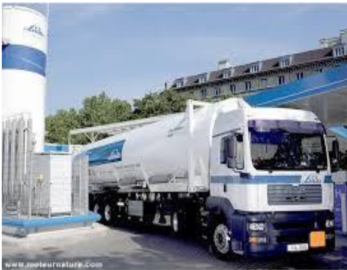
Figure 5.20 Tanker truck for transporting liquid hydrogen
