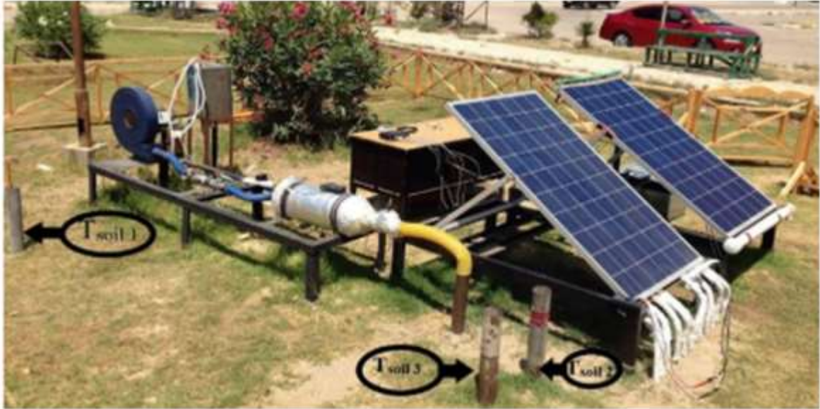
Figure (II) 6: Test stand of PV panel coupled with geothermal air-cooling system [32].
