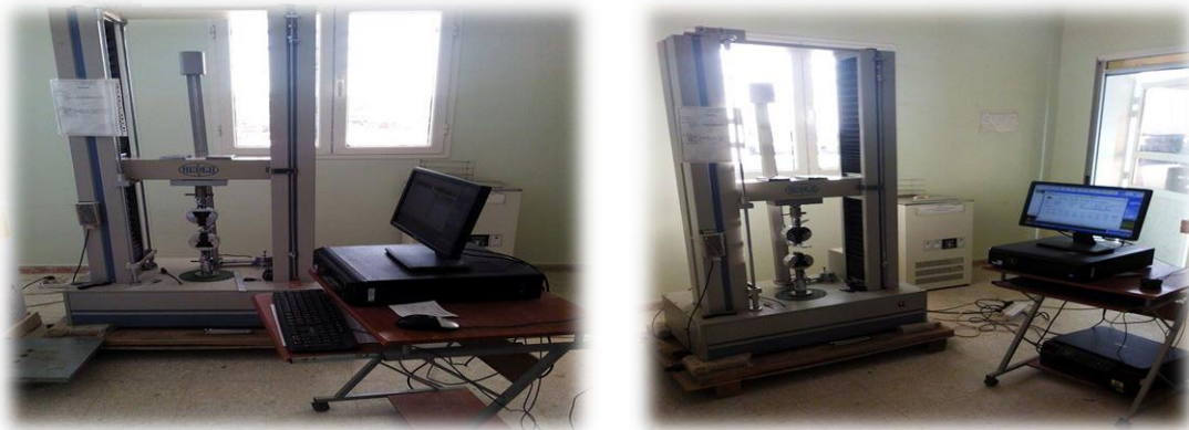
Figure (III.11): photo de la machine de traction
