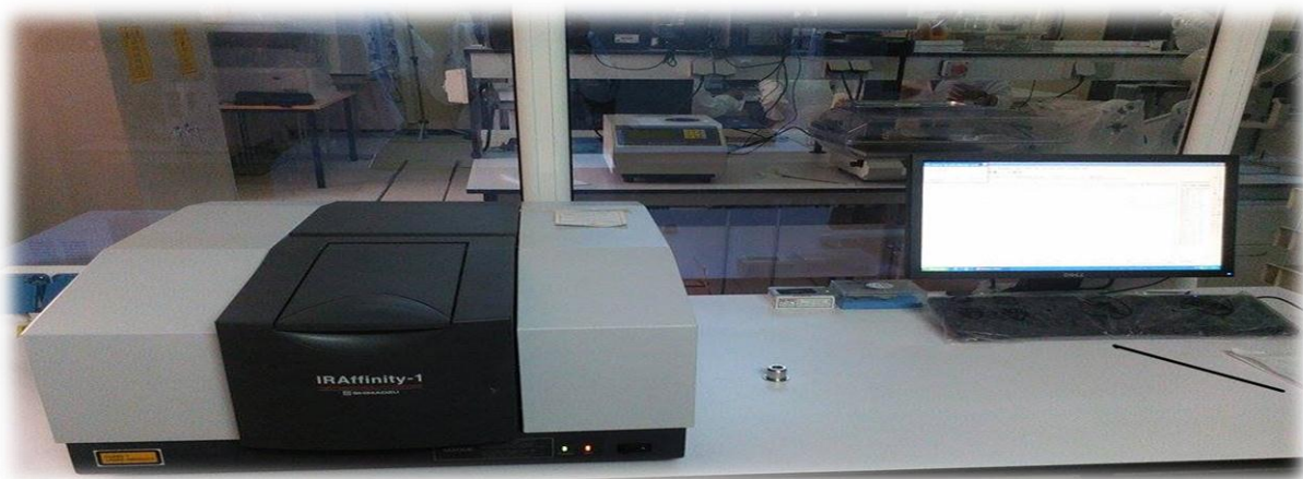
Figure (III.6): photo d'appareil IRTFFINITY-1 SHIMADZU
