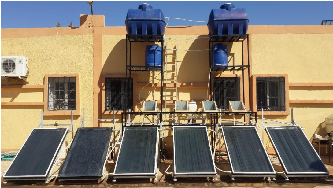
Fig.2 Photograph of the still with three FPC arrangements.
