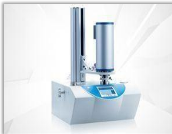
Figure II.8: Typical Thermogravimetric Analyzer (PT 1600) .
