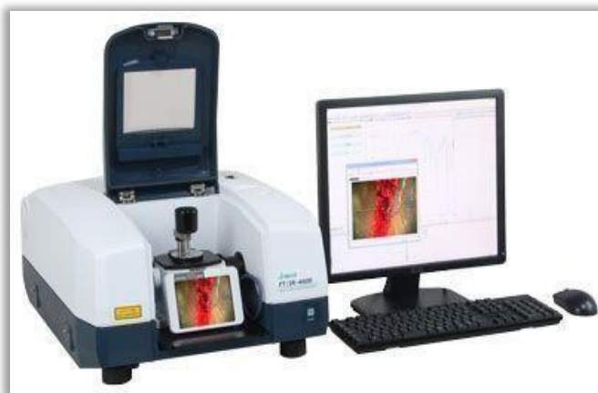
Figure II.10: Fourier transform infrared spectroscopy apparatus (FT/IR-4600).
