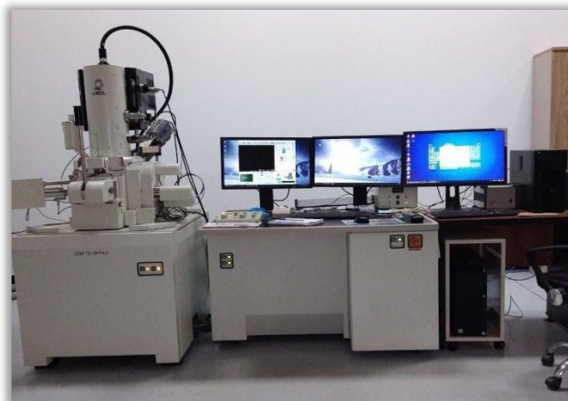
Figure II.7: Scanning electron microscope (JSM-7610FPlu).
