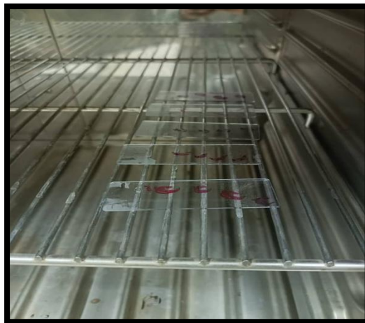
Figure 24: Placement of the slides in the oven at 60°C
