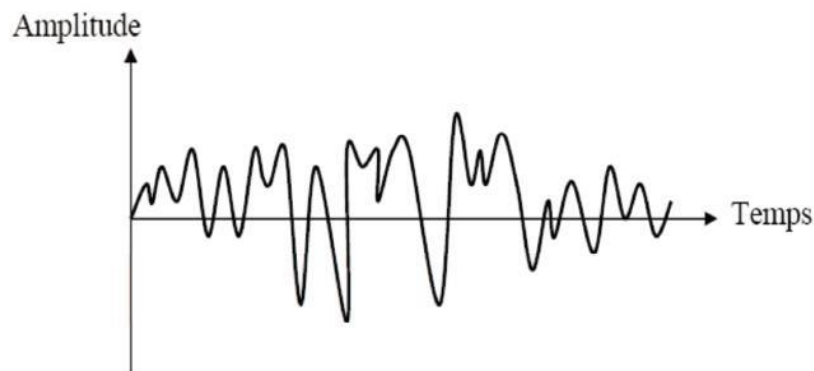
Figure II.6. Vibration aléatoire [BOU 18].
