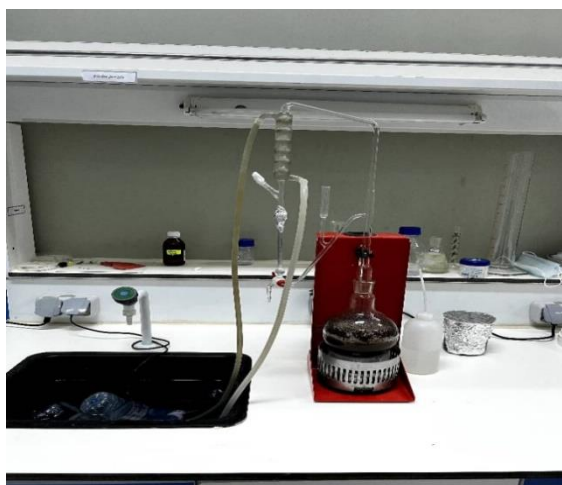
Figure 9: hydro-distillation Clevenger apparatus (Original, 2022)
