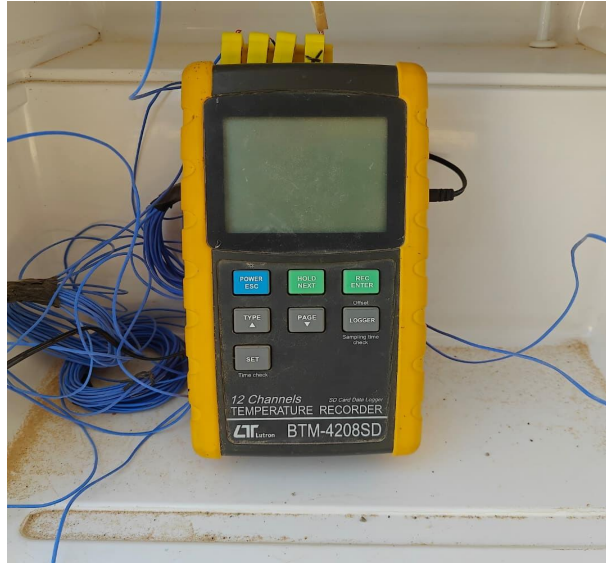
Figure 2.8: Temperature measurement device
