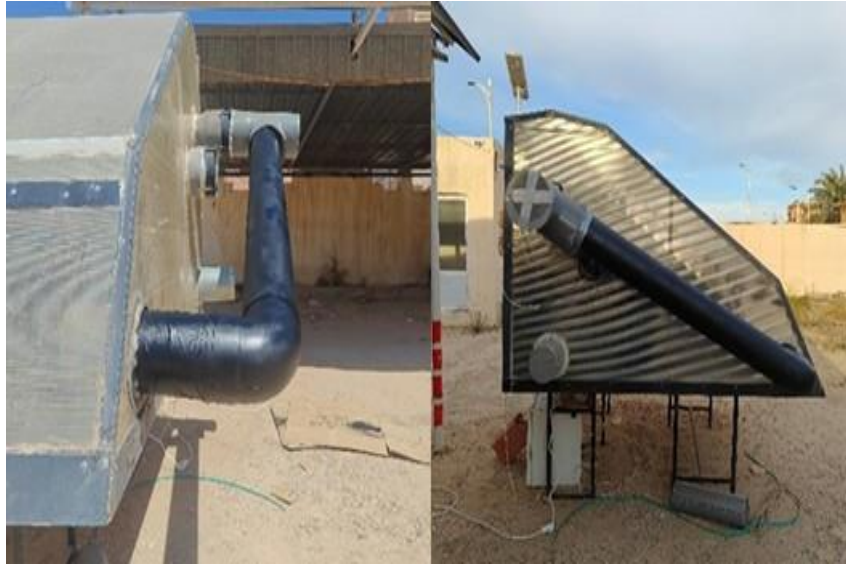
Figure 2.7: The exhaust heat recovery system with the developed greenhouse solar dryer
