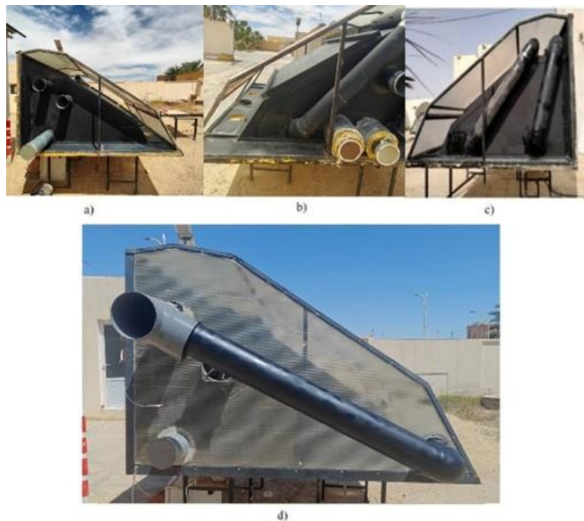
Figure 2.6: Photographs of the developed greenhouse solar dryer used in the present study
