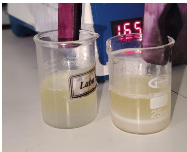
Figure 25 Phase separation appearance of moisturizing cream after thermal stress testing
