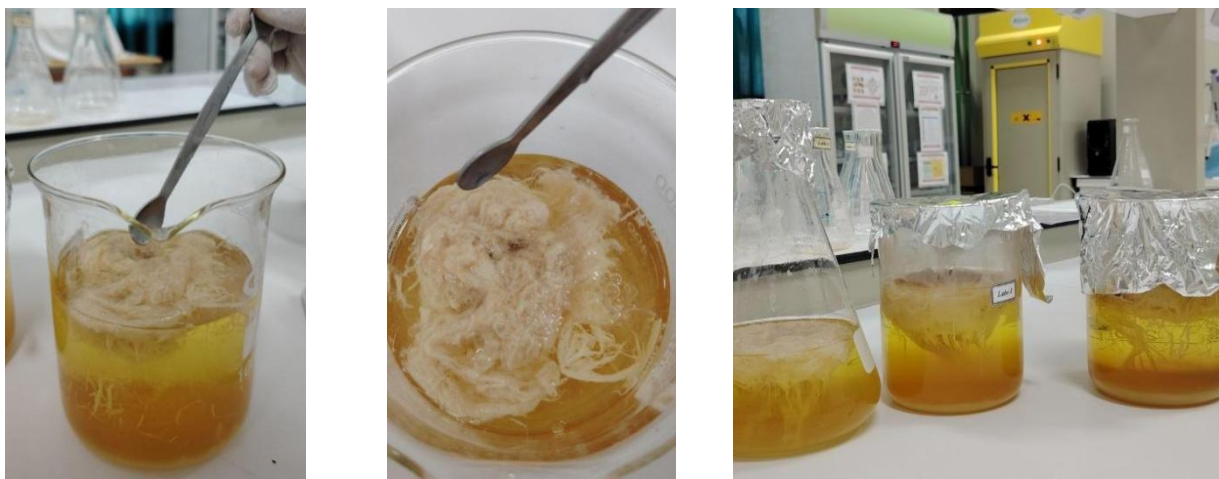
Figure.12 Precipitation of Polysaccharides (Original picture, 2026).
