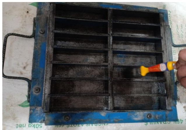
Figure II.9. Lubrification des moules.
