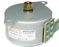
Figure III.34 : Stepper Motors M49SP-2K.
