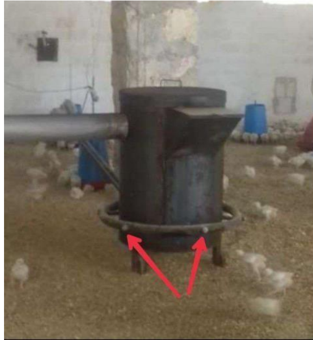
Fig II .6: The lower openings in coke burners circulate air to increase combustion. These must be cleaned regularly and carefully [40].
