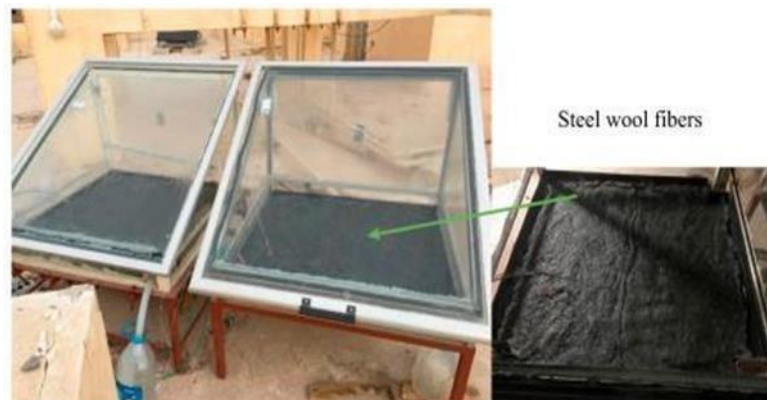
Fig. 11. A photographic of the setup of the solar still with PCM and steel wool fibers [11].
