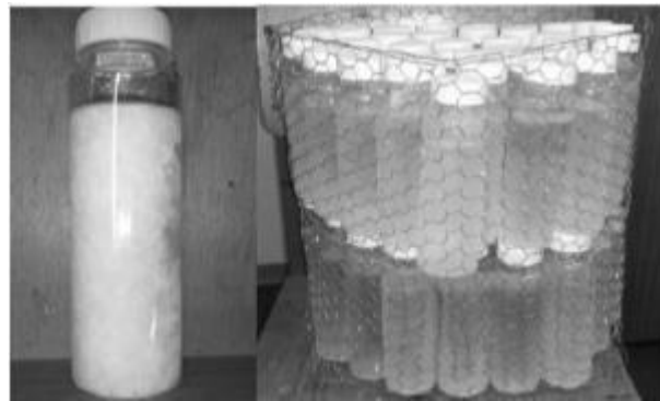
Fig. 20. Cylindrical modules inserted into storage tank [17].
