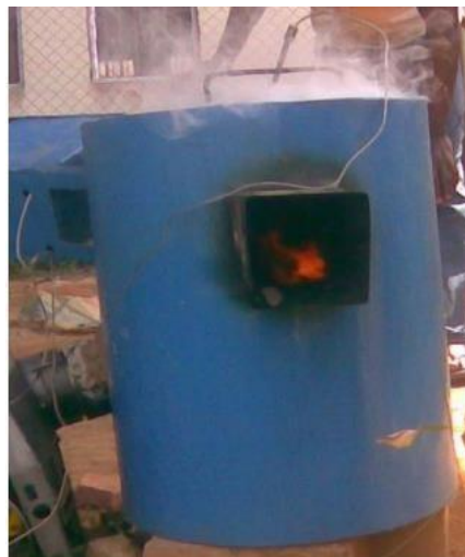
Fig II.11: The Diesel fired furnace during testing [43].
