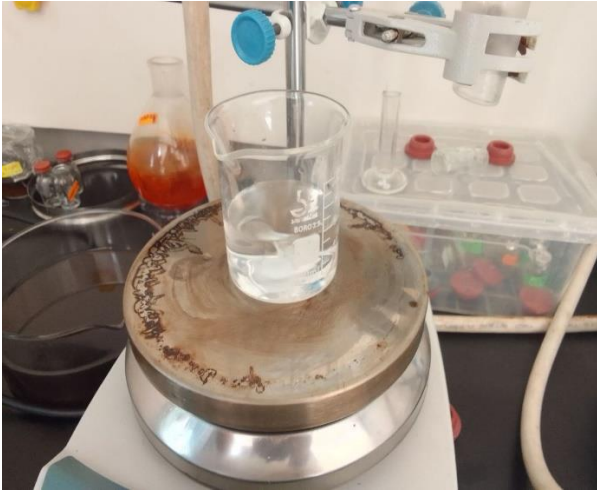
Figure 7: The synthesis of HAp by hydrothermal method
