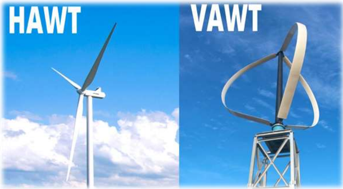
Figure I. 1: The two types of wind turbines in terms of the way they rotate and the difference between them[22]
