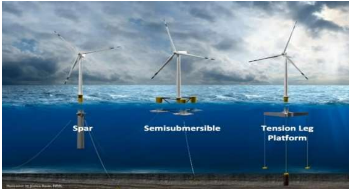
Figure I. 9: Floating platform concepts for offshore wind turbines[38]
