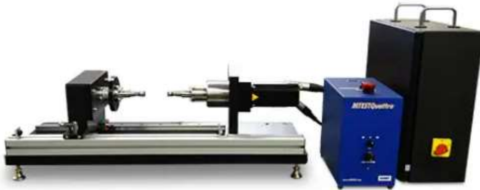
Figure I. 11: Torsional stress testing machine[45]
