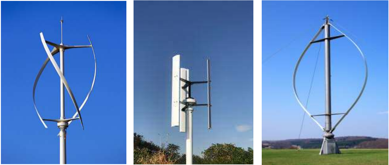
Figure I. 4: Types of Darrieus wind turbines[31]
