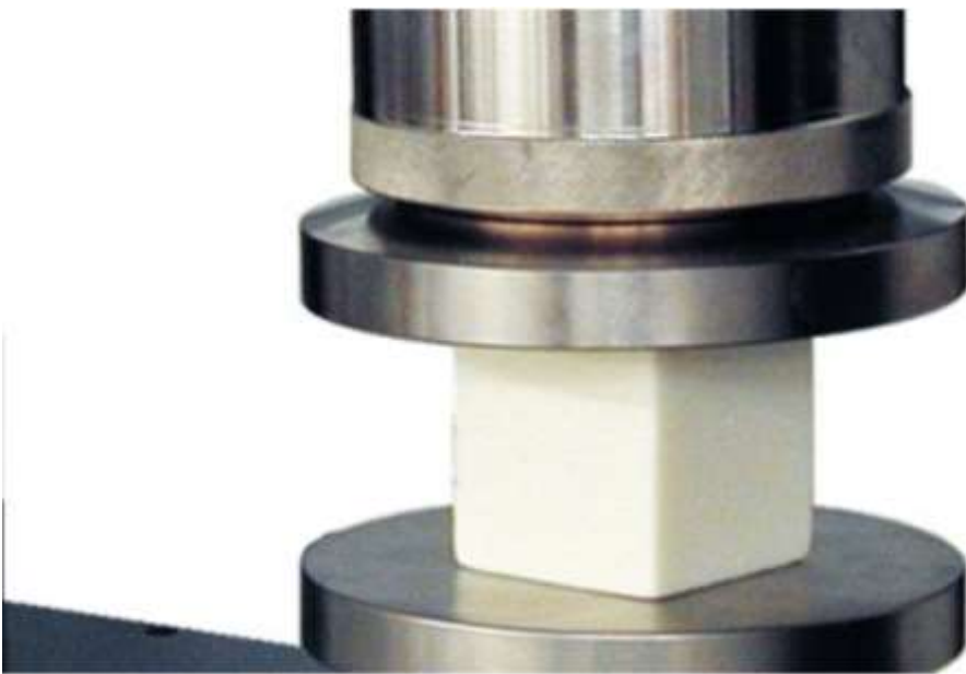
Figure I. 14: Pressure testing machine[45]
