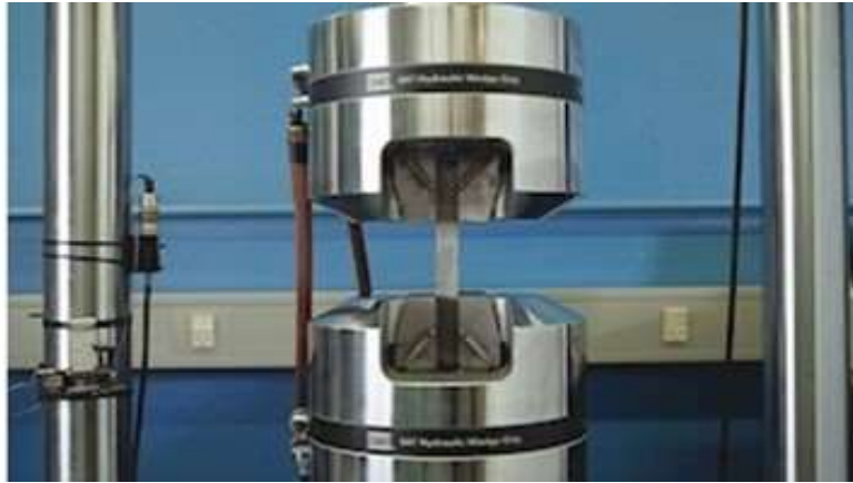
Figure I. 15: Fracture mechanics testing machine[45]
