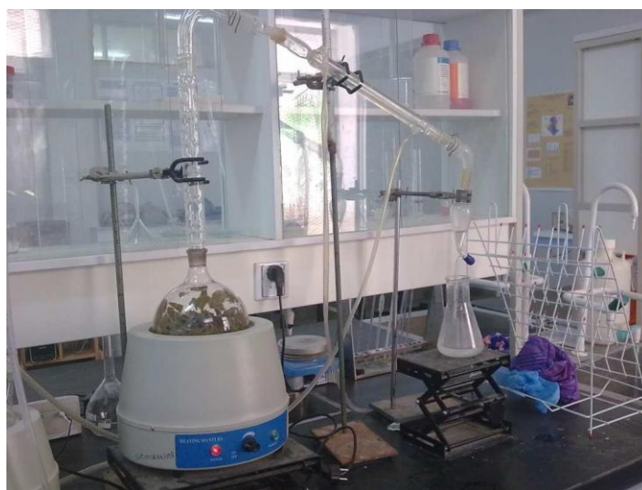
Figure 9 : Hydrodistillation (Clevenger) (AYAIDIA., 2011).
