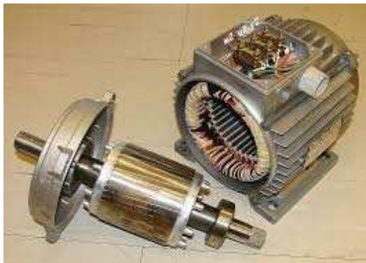
Fig I.1: Machine asynchrone: stator et rotor.
