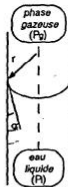
Fig. 4.8 Schematic representation of a meniscus in a capillary.
