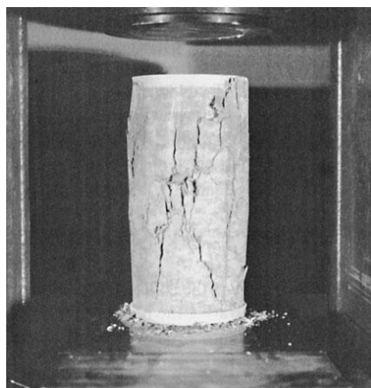
Figure 4-2: Typical failure mode of concrete under compression.
