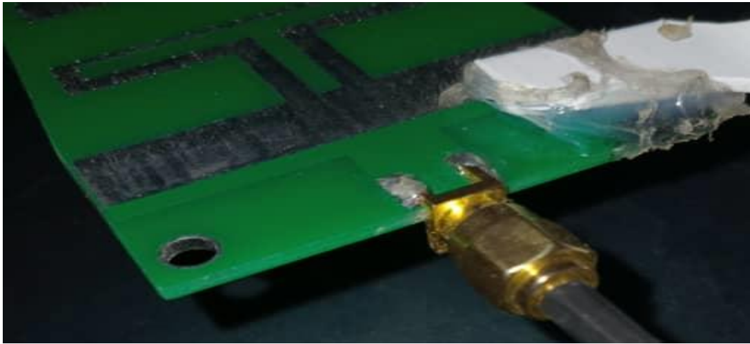
-Figure 13: NRF with an SMA male to SMA female cable to the Yagi –
