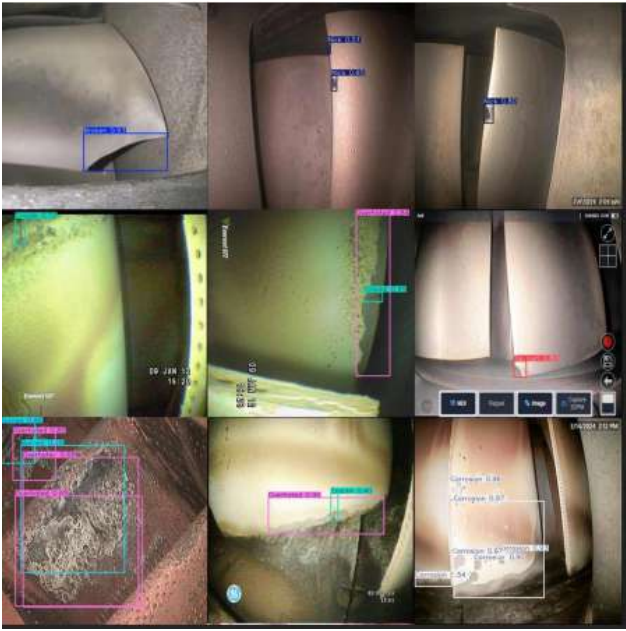
Figure III.18: Obtained results of damages detection by the proposed approach: Yol11 model on testing images
