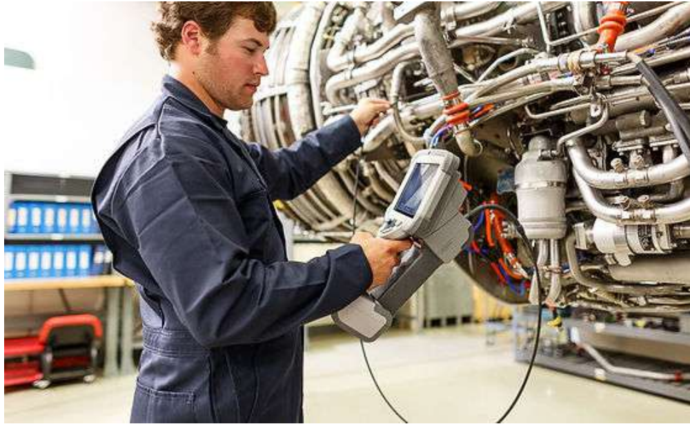
Figure II.5: Aircraft Engine Inspection by Maintenance Technician Using a Borescope[15]
