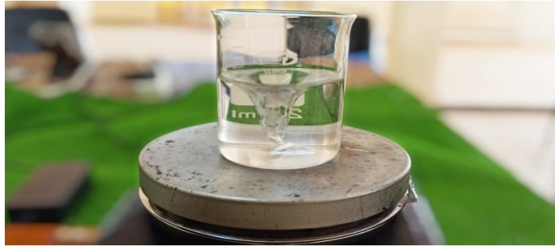
Figure III.33: Testing the effectiveness of mixing operation in the device.
