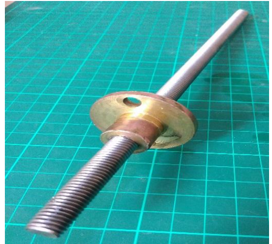
Figure 21. Vis de transmission
