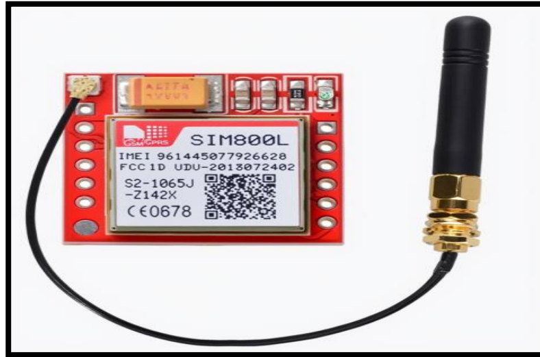
Figure II.10: Example of a SIM800L cellular communication module.
