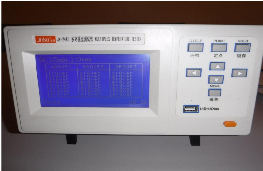
Figure (III.9): multiplex temperature tester
