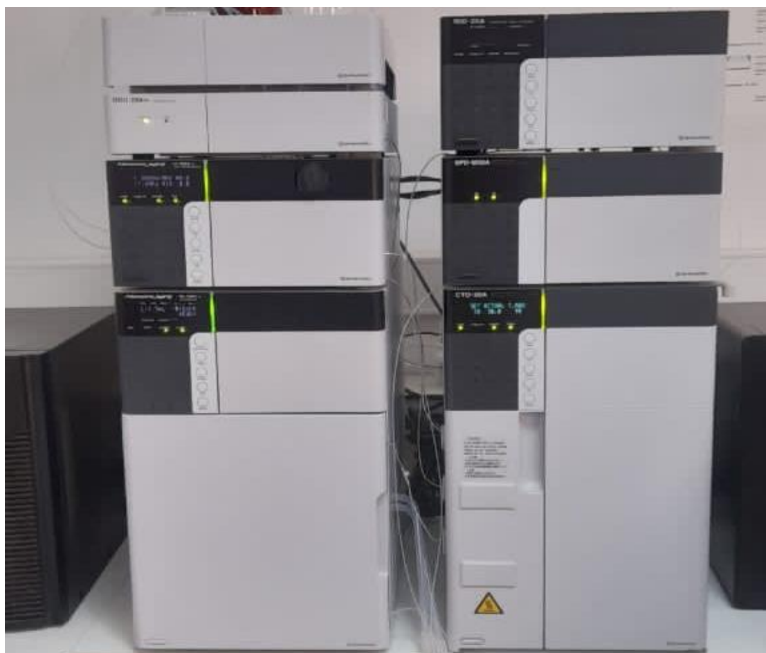
Figure : High performance liquid chromatography device HPLC
