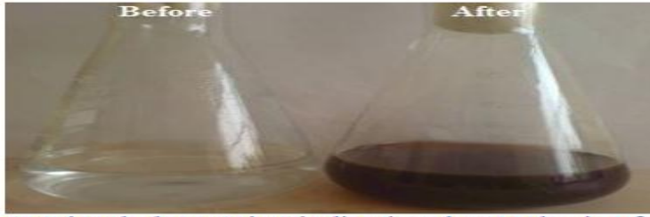
Fig. 1: Visual observation indicating the synthesis of silver nanoparticles using Foeniculum vulgare seed extract.
