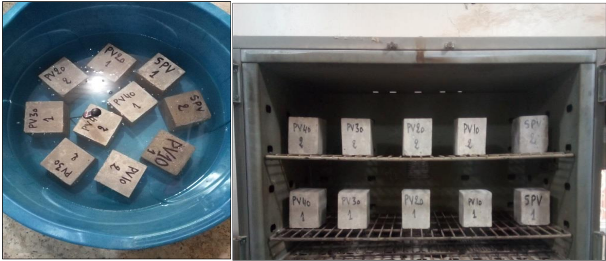
Figure II.21. Essai mouillage - séchage.
