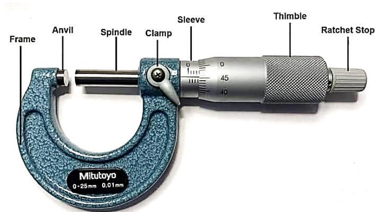
Figure 21: The components of the external micrometer gauge
