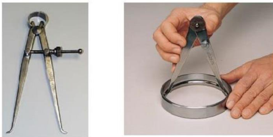
Figure 8: Outside calipers and uses
