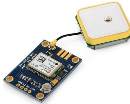
Figure 2.9: Global Positioning System (GPS) Module Used in Drone Systems
