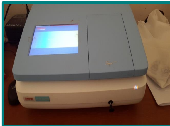
جهاز UV-Visible طراز Spectrum Instruments/ SP-UV 300 SRB
