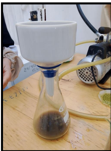
Figure 4. 6 Vacuum Filtration Using Filter Paper
