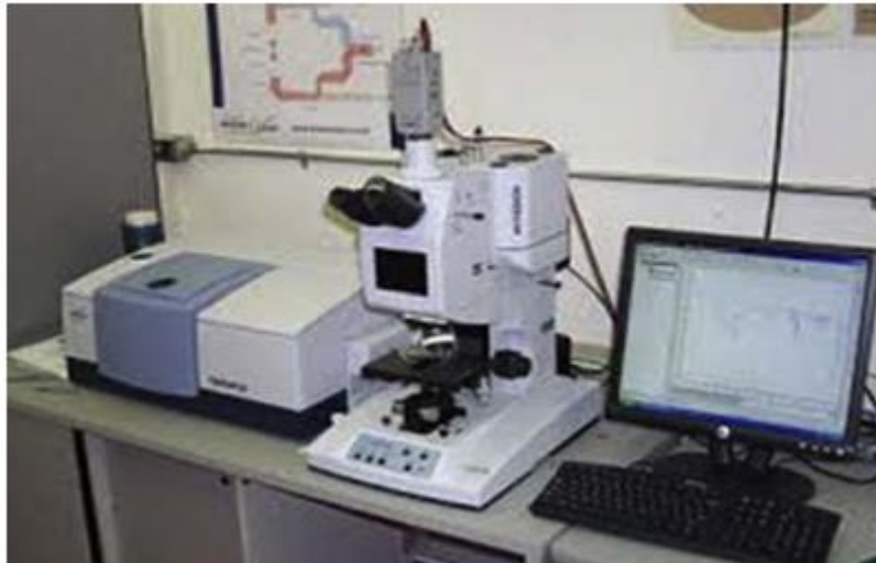
Figure 3. 3 Fourier transform infrared instrumental setup[14]
