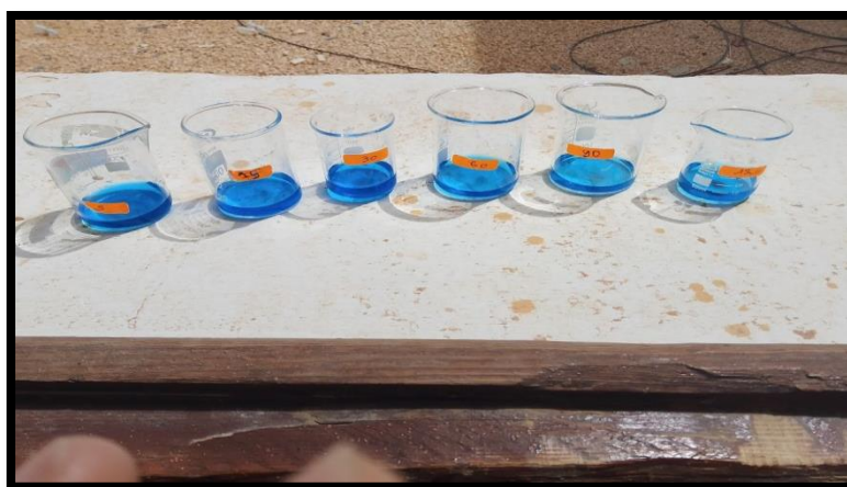
Figure 4. 23 Sunlight irradiation of Methylene Blue dye samples in the presence of ZnO nanoparticles
