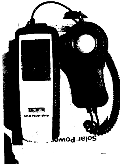
Fig III.8 Solar power meter
