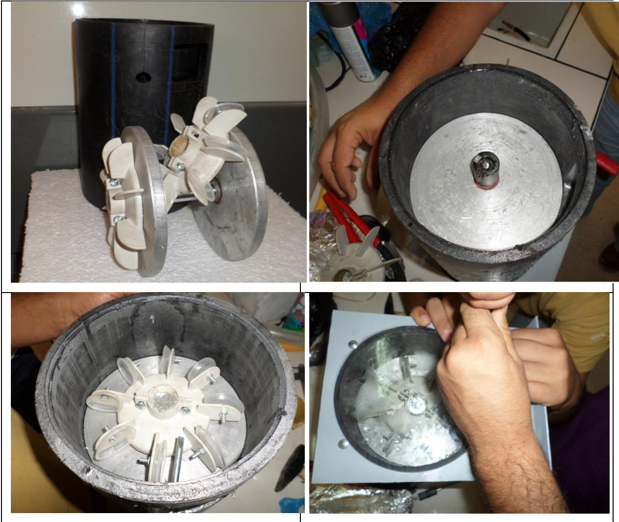
Figure II.4 montage de la turbine
