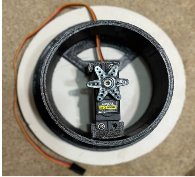
Fig III.19. Servomotor assembled on the base.
