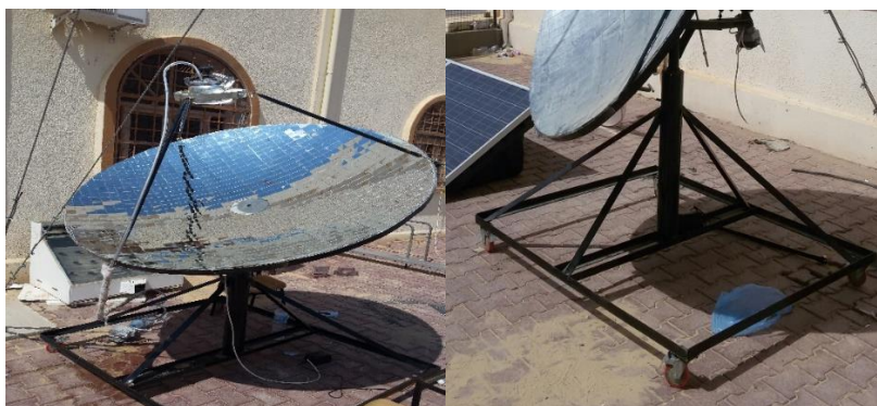
Figure III.3: Le support de concentrateur
