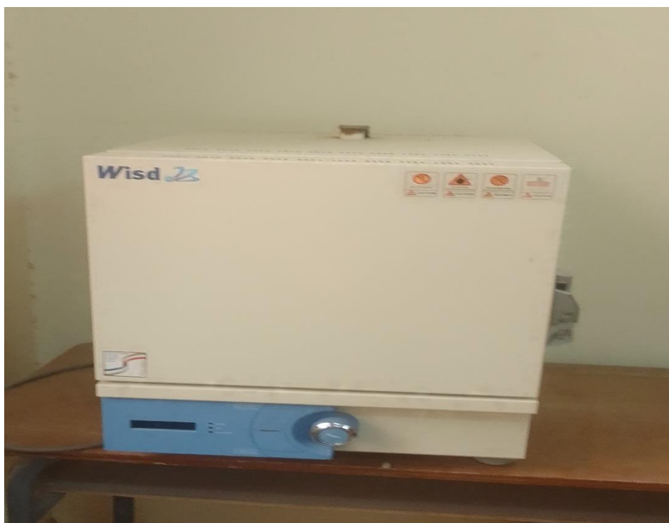
Figure 14: High temperature high treatment furnaces
