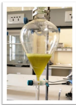
Figure 05: Separation by separatory funnel of Ephedra extract
