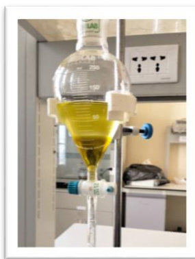
Figure 04: Separation by separatory funnel of Lavender extract
