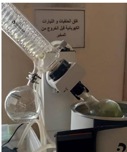
Figure 09: Drying step by rotavapor
