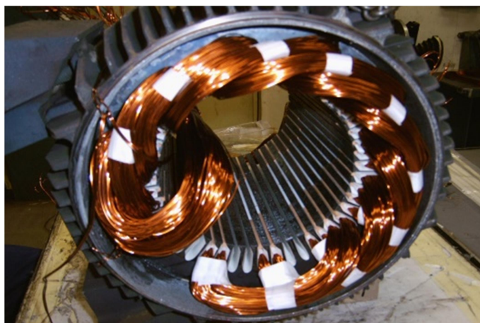
Figure (I.1) : Stator de la machine asynchrone.
