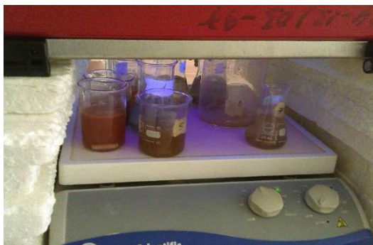
Fig.9. Test of photodegradation ( Vat Green 03 textile dye ) of the mixtures ( \text{TiO}_2 + \text{DB} ) and ( \text{TiO}_2 + \text{DMF1} ) in the photocatalytic reactor ( transilluminator )
