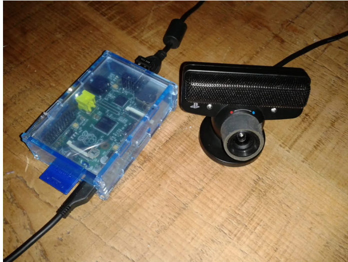
FIGURE 3.18: Physical Assembly of Facial Recognition Subsystem with Raspberry Pi and Webcam.
