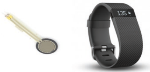
Figure 1.4: Examples of pressure sensors. (Source: Force Sensing & Fitbit)
