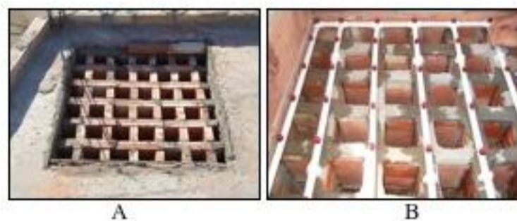
Fig.2. Horizontal cross-section of the wind tower 1 \times 1 \text{ m}^2 with partitions of 10cm in section and a total number of 49 conduits (A), water spray pipes (B)
