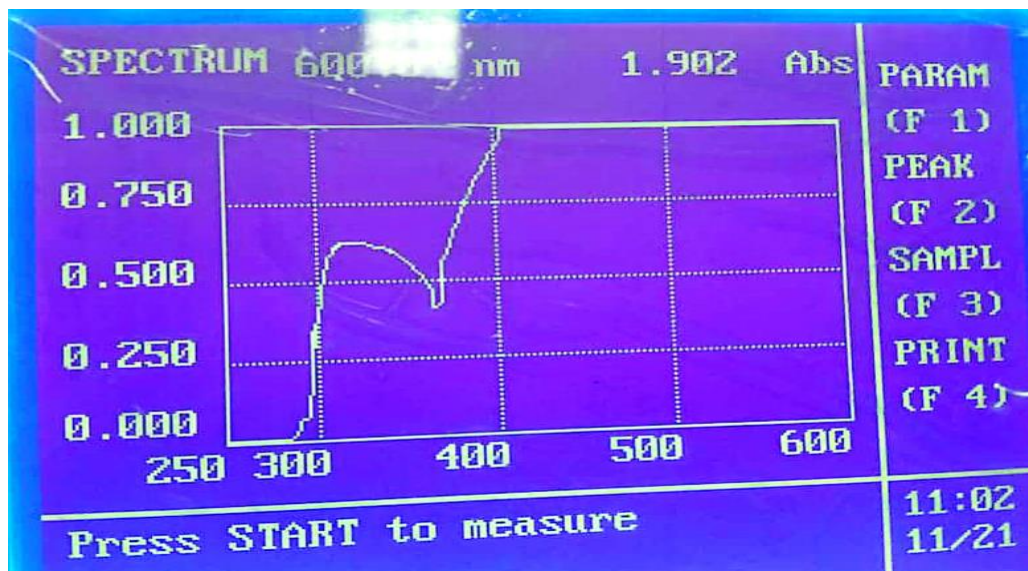
Figure 11: UV-Vis spectra of copper oxide nanoparticles.
