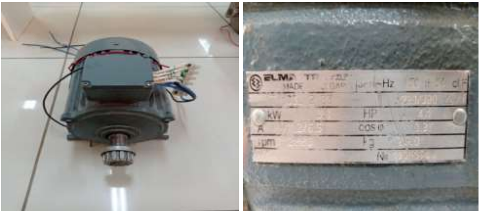
Figure (II. 16): Three-phase induction machine 1.
