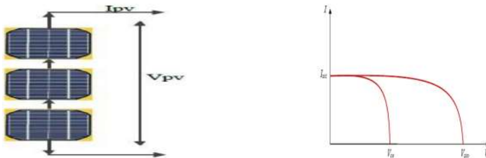
Figure (I. 4): Characteristics of series-connected solar cells.
