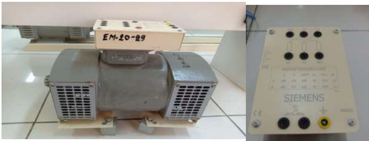
Figure (II. 15): Three-phase synchronous machine.
