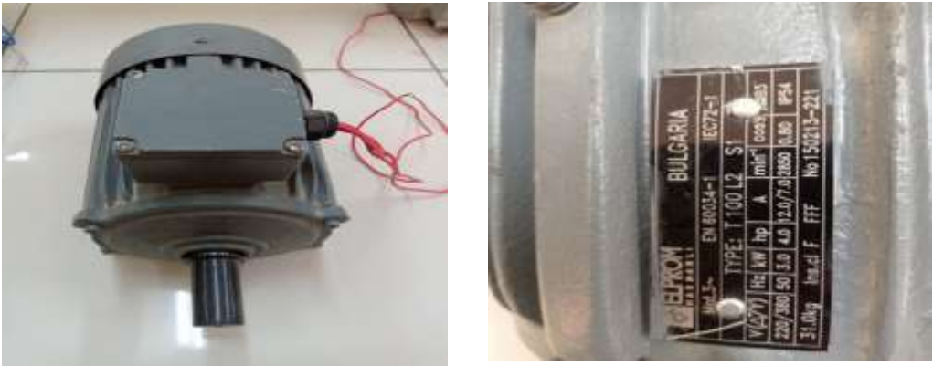
Figure (II. 17): Three-phase induction machine 2.
