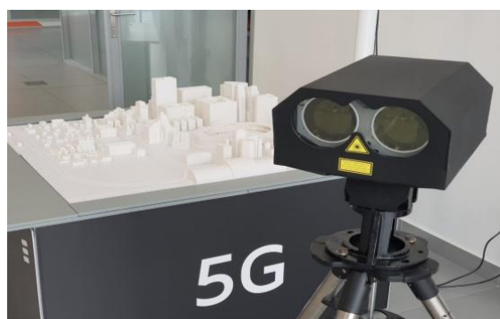
Figure 1.5: Advanced FSO Transmitter with Beam Alignment Technology.
