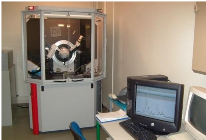
Figure II.3: Diffractomètre de marque Advanced Bruker D8.
