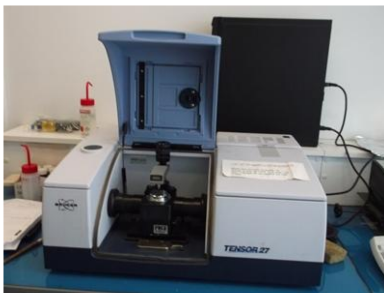
Figure II.7: Appareil FTIR de marque TENSOR 27.
